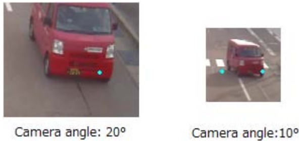
Figure 7. The images extracted from videos of different camera angles for the same car
