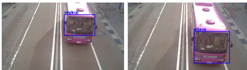
Figure 6. Multiple counting for the same vehicle at the angle setting of 30 degrees (left: detected by the left down lane; right: detected by the right lane again )
